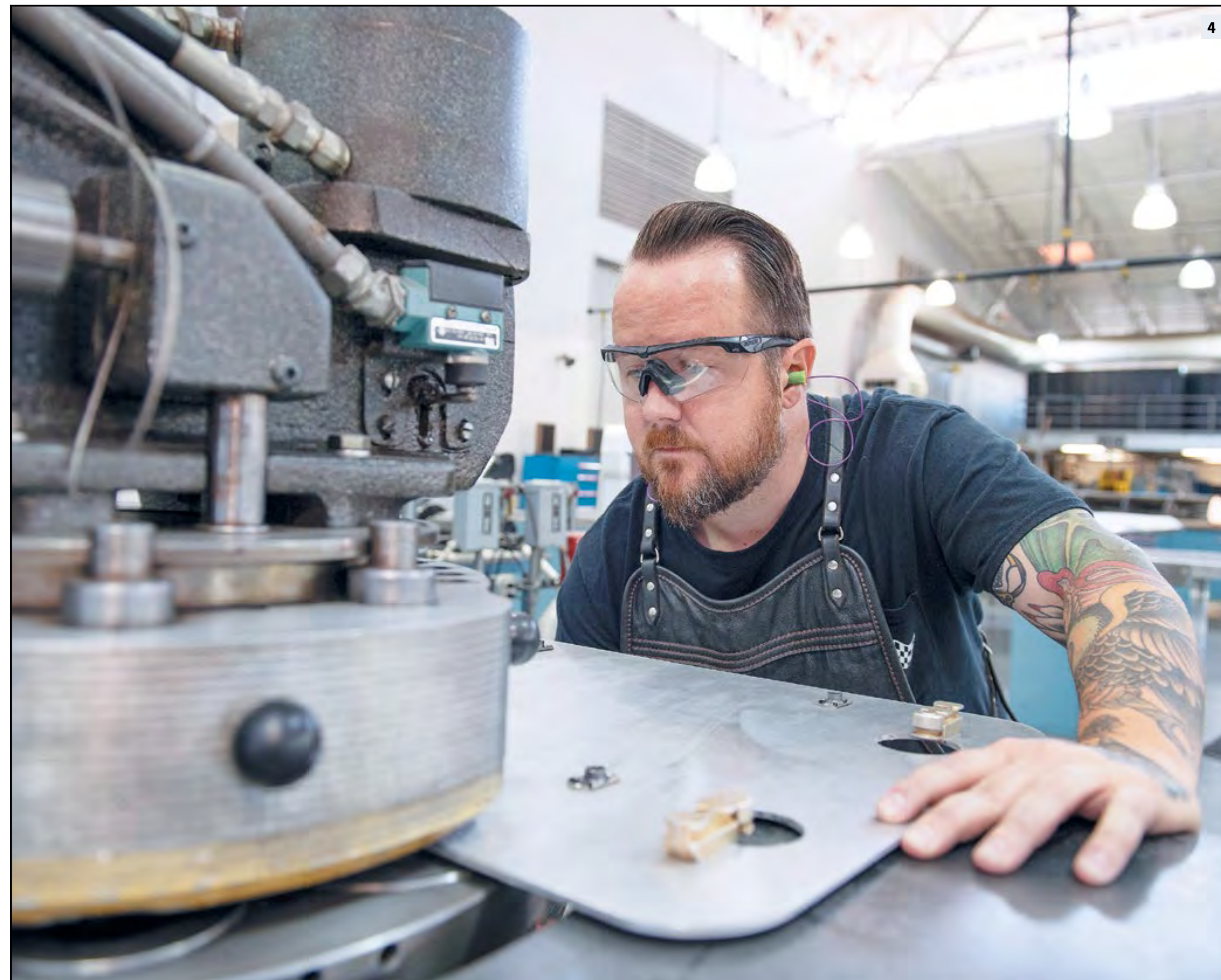
1) Tech. Sgt. Zachary George, 60th Air Mobility Wing Phoenix Spark Lab noncommissioned officer in charge, looks at a plate he helped design June 25 at Travis Air Force Base, California. The plate will securely attach a GSA-approved safe to the floor of a KC-10 Extender, which will allow aircrew members to store weapons and other sensitive materials on the aircraft. 2) George works with computer animation software to design a safe June 25 at Travis AFB. George designed the plate that will securely attach a GSA-approved safe to the floor of a KC-10 Extender, which will allow aircrew members to store weapons and other sensitive materials on the aircraft. 3) George installs a fabricated plate on the floor of a KC-10 June 27 at Travis. 4) Jeffrey Bruns, 60th Maintenance Squadron sheet metal shop template maker, cuts holes into a plate June 25 at Travis AFB.
